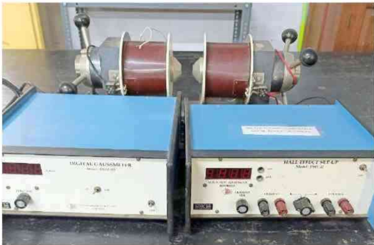
Hall Effect - Experimental Set-up
